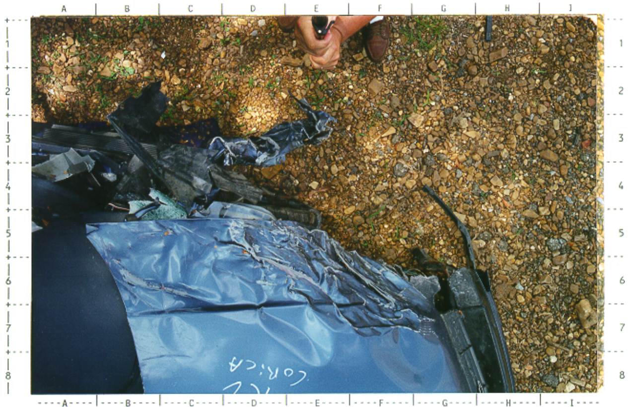
# 39 -- Overhead left front view of crush to 1991 Chevrolet Corsica's left front fender crush
